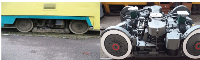
Figure 2 – Tatra RT6N1 (a), Tatra 3 (b) tram trolley equipped with a mechanical brake on the engine shaft and a rail electromagnetic brake
